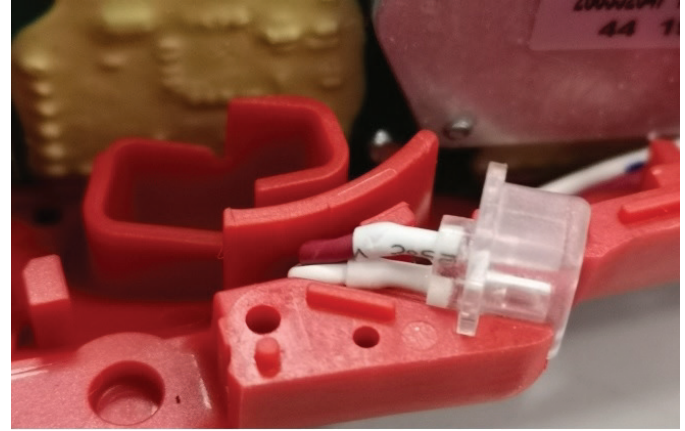
4. Place LED light in recess with the red wire to the top
