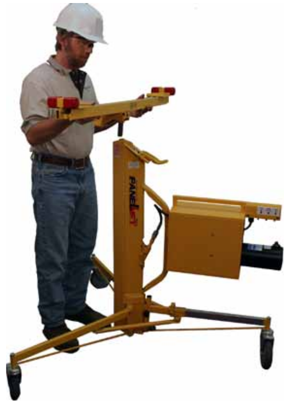
10. MOUNT THE CRADLE ON TOP OF THE TELESCOPING SECTIONS. PULL OUT ON THE TILT LATCH TO ALLOW THE CRADLE TO TILT FOR LOADING AND FOR HANGING DRYWALL ON SIDEWALLS AND SLOPED CEILINGS.
