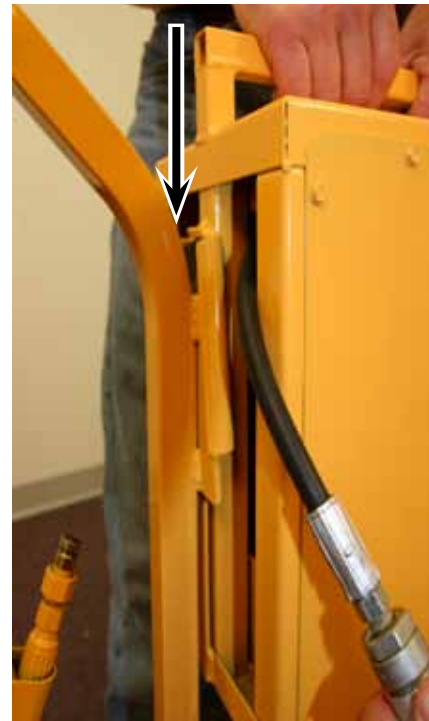
6B. SLIDE THE POWER BOX DOWN MAKING SURE THAT THE TAPERED PLATE AND TAPERED SLOT ALIGN UNTIL THE PLATE BOTTOMS OUT AND LOCKS IN PLACE.
