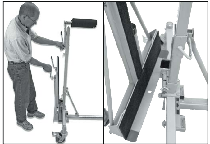
5. Hang carrier on storage pin and fasten to frame with storage latch pull pin.
