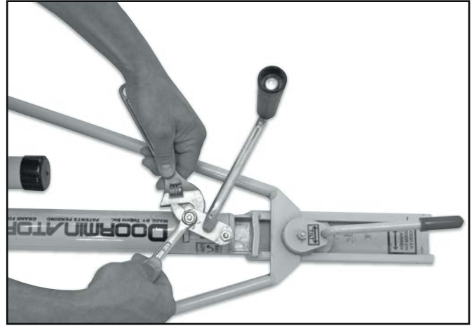
4. Bolt on crank handle to door carrier.
