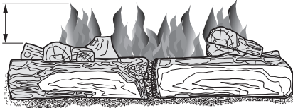
Figure 32 - Correct Burner Flame Pattern
