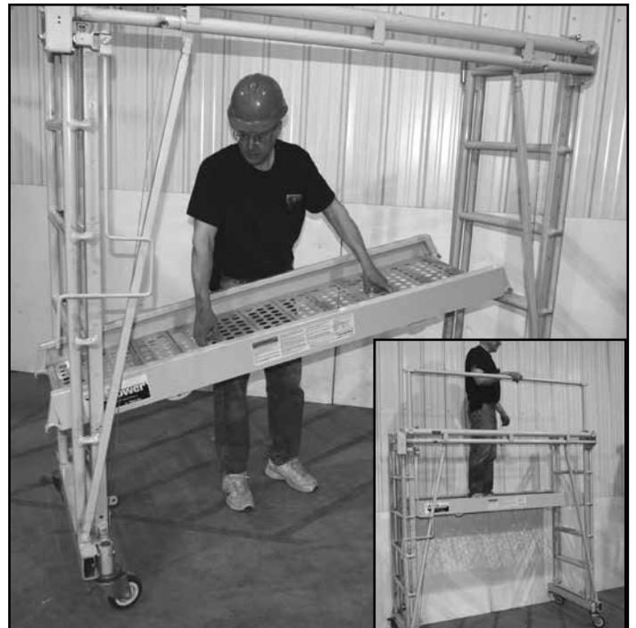
8) For platform heights from 2' to 6', the deck may be placed on lower rungs. For added safety use guard rails even when deck is on lower rungs.
