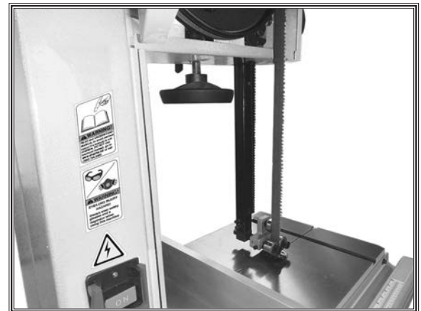
Figure 95. Guide post guard removed.
