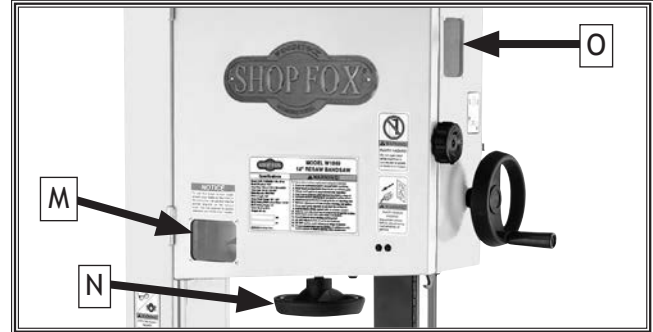
Figure 5. Blade tension scale, blade tension handwheel, and tracking window.
