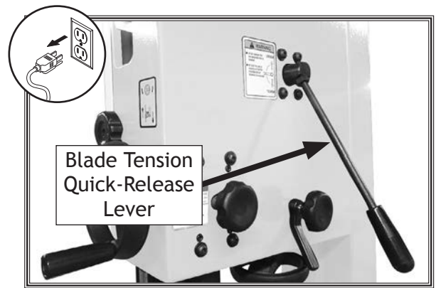
Figure 33. Quick-release blade tension lever in down position, applying tension to blade.
