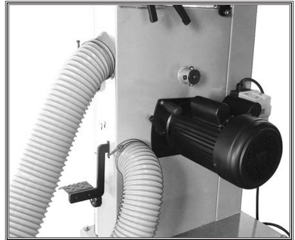
Figure 31. Example of dust hoses attached to upper and lower dust ports.
