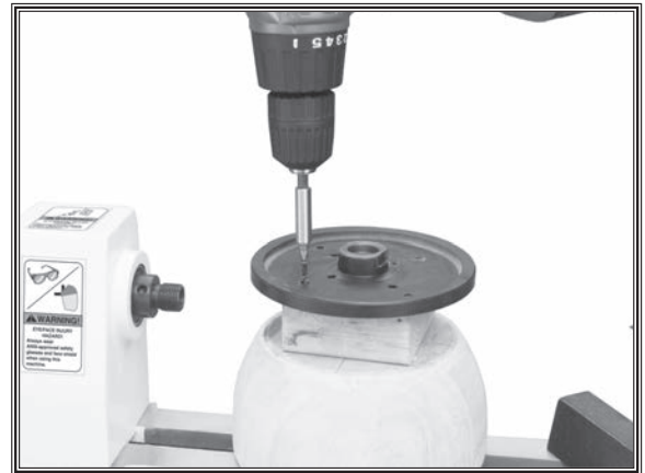
Figure 32. Example of attaching faceplate to workpiece.
