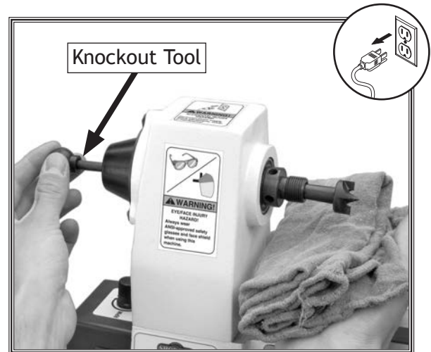
Figure 21. Removing center from headstock spindle with knockout tool.
