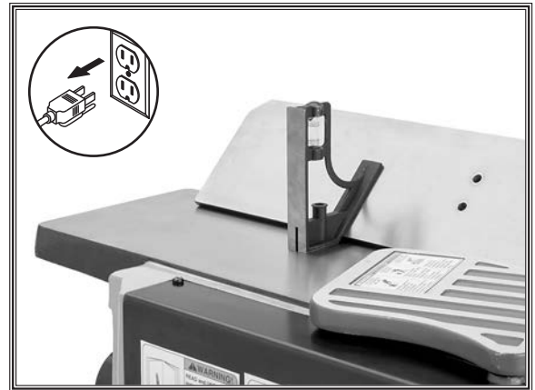
Figure 47. Checking the outward 45° stop.
