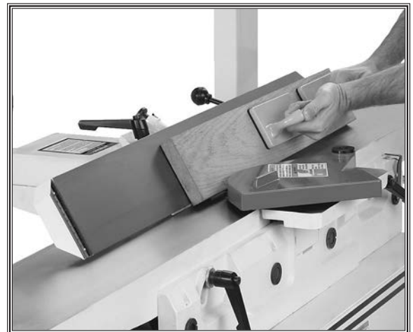
Figure 35. Typical bevel cutting operation.
