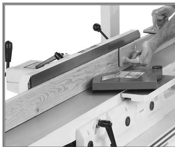
Figure 33. Typical edge jointing operation.
