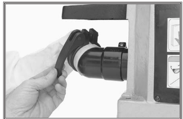
Figure 17. Attaching the dust collection bag.
