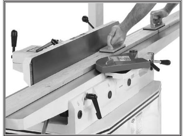
Figure 30. Typical surface planing operation.
