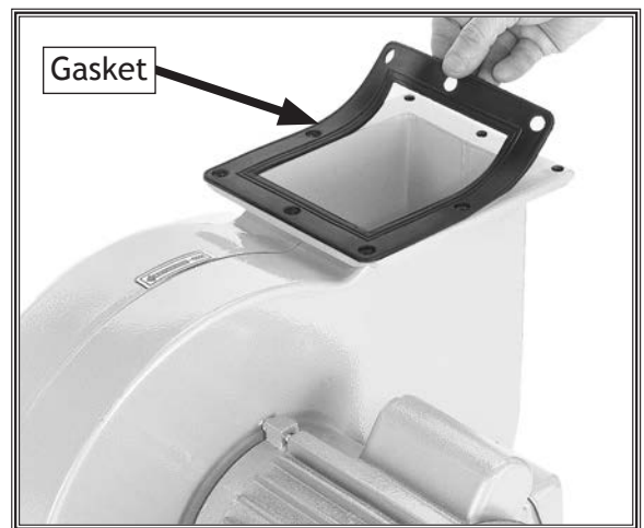
Figure 8. Positioning impeller outlet gasket.
