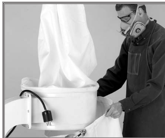
Figure 42. Replacing lower bag.
