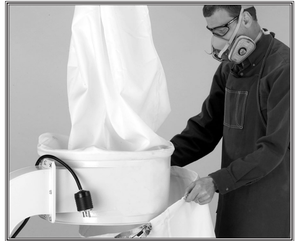
Figure 38. Replacing lower bag.
