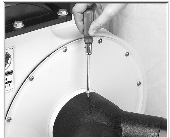
Figure 17. Attaching inlet Y-connector.
