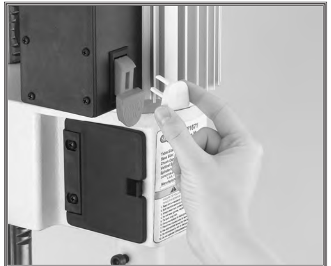
Figure 5. Remove safety key when not in use.
