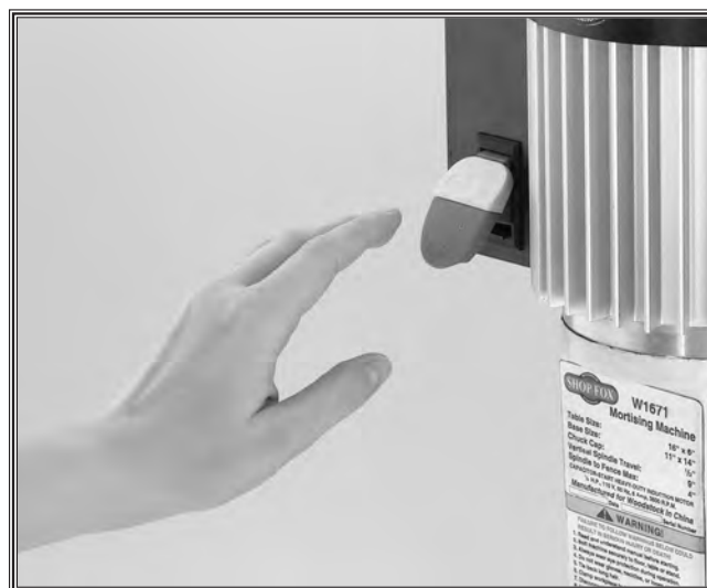
Figure 30. Hand poised over stop paddle.
