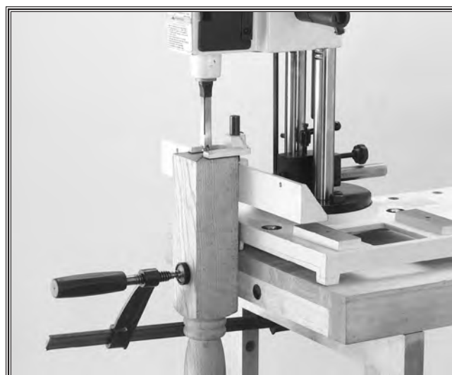
Figure 24. Workpiece clamped to edge of table.
