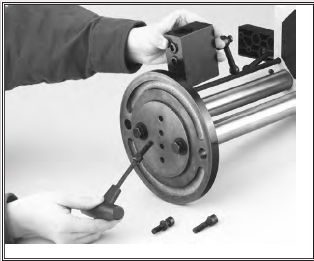
Figure 28. Repositioning the support block.
