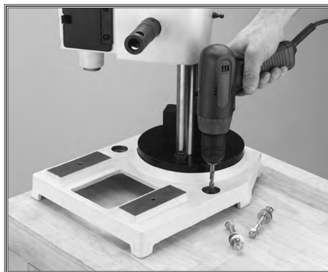
Figure 10. Using mounting holes as drill guides.
