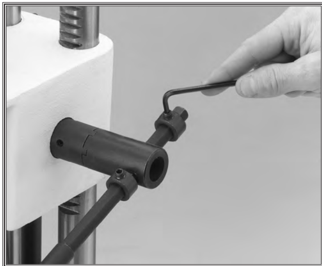
Figure 11A. Secure collar onto hand lever.
