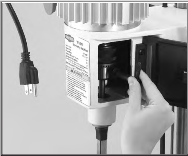
Figure 2. Unplug before changing chisels.
