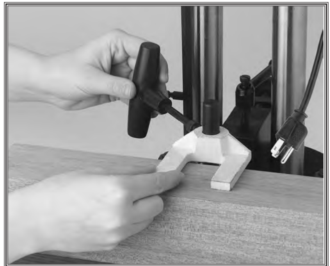
Figure 3. Always clamp workpiece.
