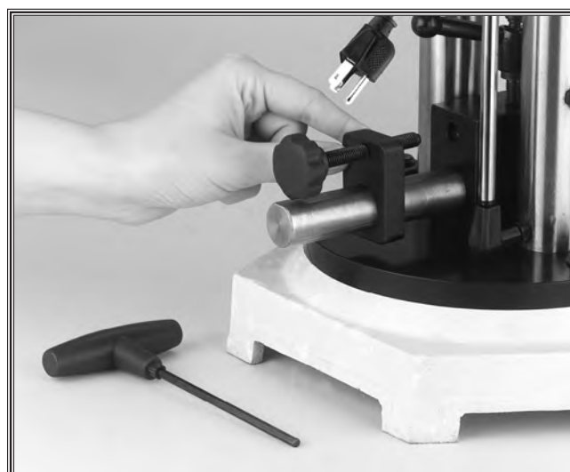
Figure 26. Setting micro-adjusting block.
