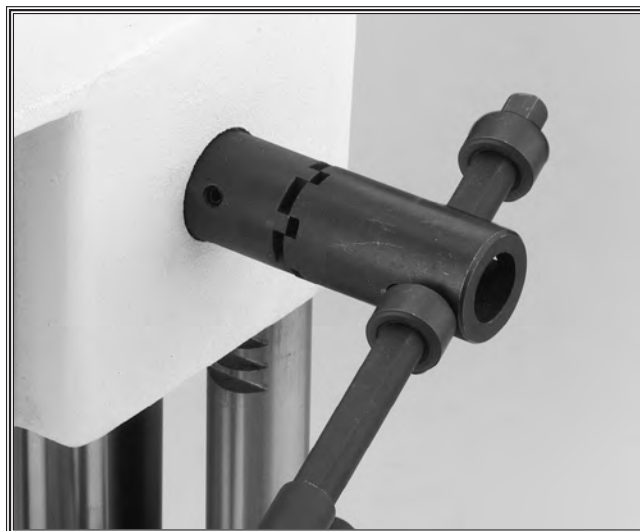
Figure 12. Indexing handle by swinging out.
