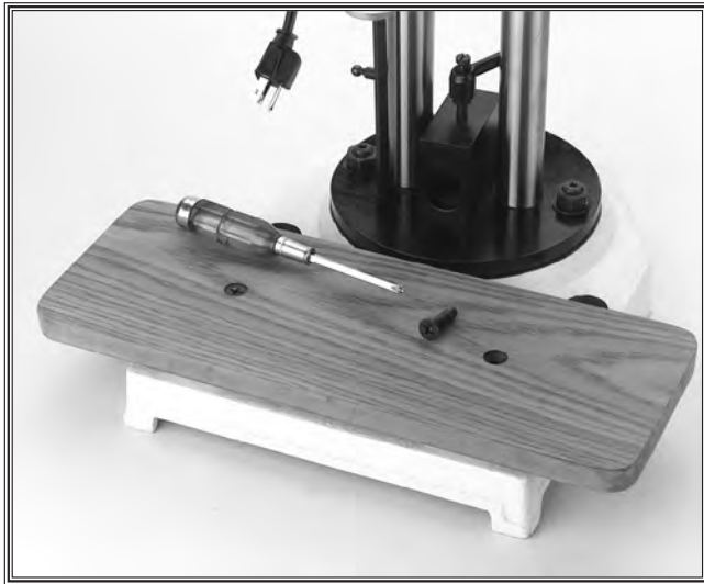
Figure 14. Work table secured with screws.
