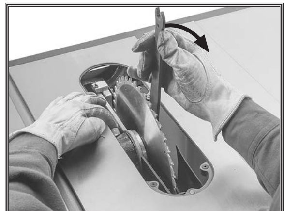
Figure 48. Example of removing table saw blade.
