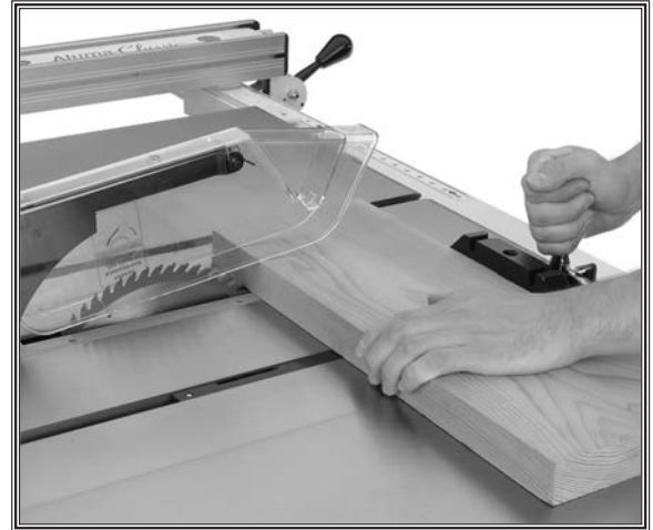
Figure 61. Typical crosscutting operation.
