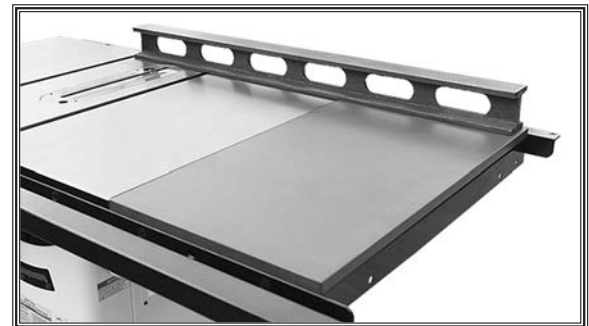
Figure 28. Adjusting extension table flush with wing and table.
