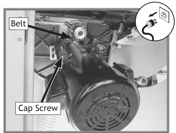
Figure 128. Location of cap screw for adjusting belt tension.
