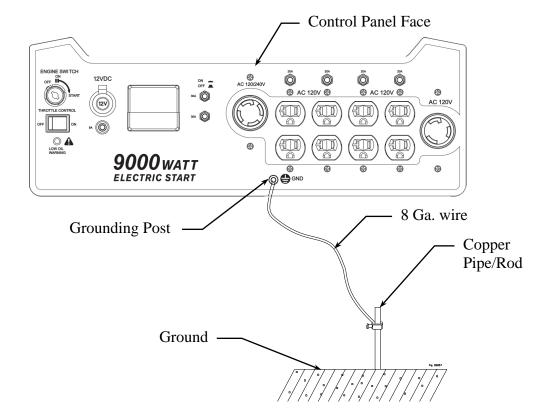
If a licensed electrician installs the generator with a connection to your buildings electrical circuit for use as a back-up power system, grounding may alternatively be completed through the building's grounding system. Ask your electrician. If the generator is not grounded through your building's electrical system, follow the procedure above.
