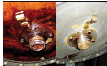
Vessel cover contaminated
