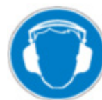
Loud Noise Hazard - Wear Ear Protection
