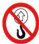
Do Not Lift Equipment with Hook - No Lift Point
