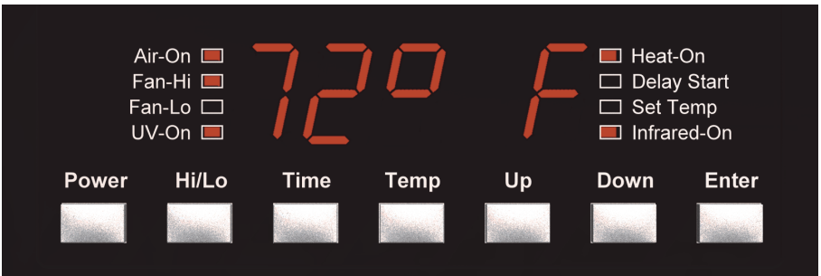
LED Display and Control Panel for Setting the Temperature
