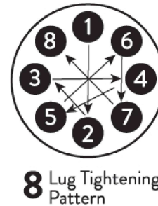
Figure 3 - Recommended 8 Bolt Tightening Pattern (STAR)
