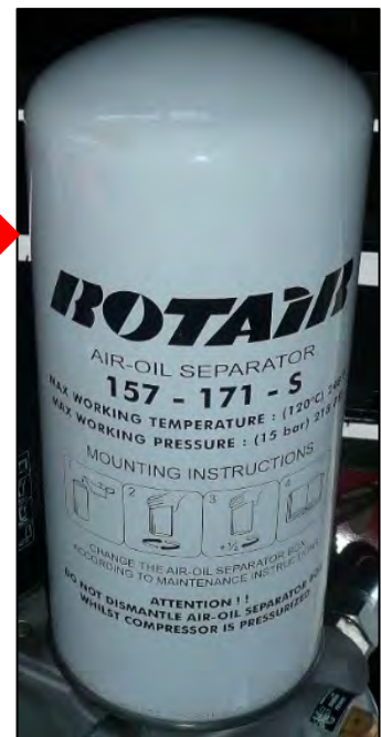
Figure 13.4-7 Oil separator filter
