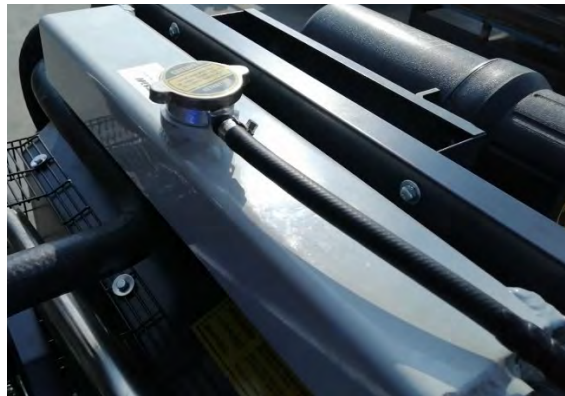
Figure 10.1-3 Checking the radiator cooling liquid
