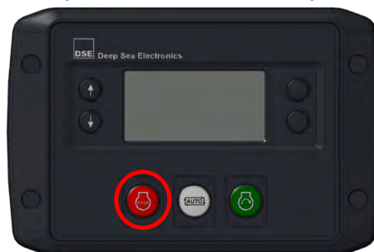
Figure 8.3-1 STOP button on the electronic board deepsea
