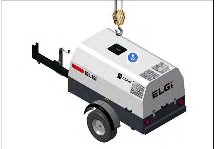
Figure 6.2-1 Instruction for lifting procedure
