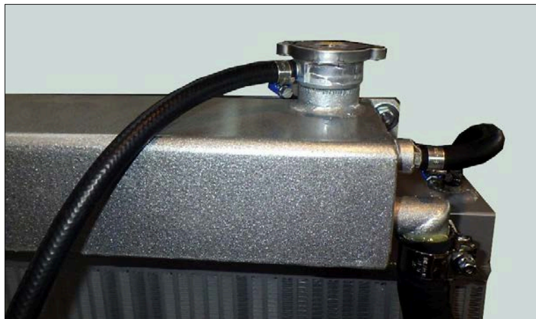
Figure 13.4-3 Checking the coolant radiator
