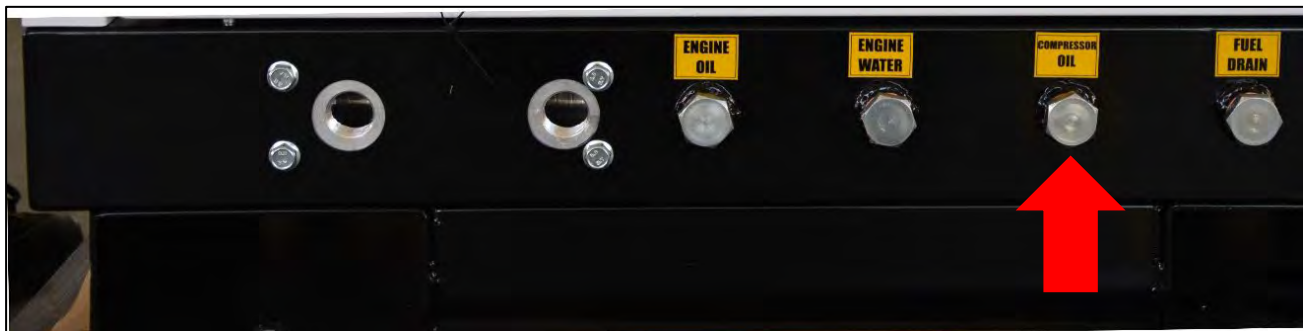
Figure 13.4-8 Compressor oil drainage
