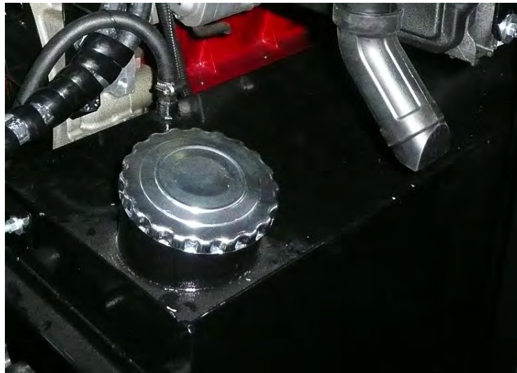
Figure 10.1-1 Gas oil tank for Diesel engine
