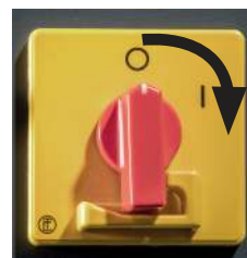
Switching on the power switch
