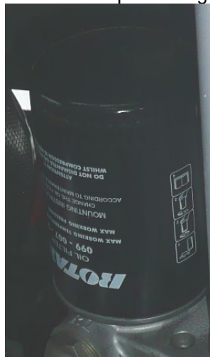
Figure 13.4-6 Compressor oil filter
