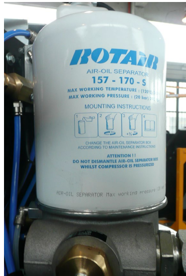
Figure 13.4-7 Oil separator filter
