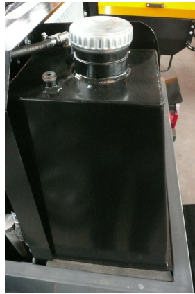
Figure 10.1-2 Fuel tank for Diesel engine
