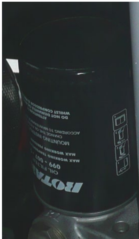
Figure 13.4-7 Compressor oil filter
