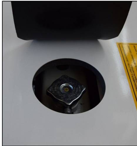
Figure 13.4-2 Checking the coolant radiator
