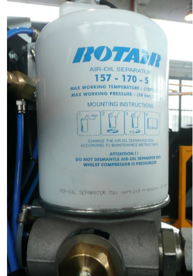
Figure 13.4-7 Oil separator filter
