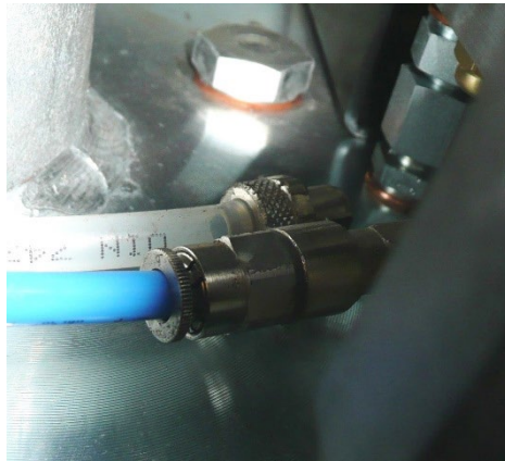
Figure 13.4.7-1 Nozzle oil recovery
