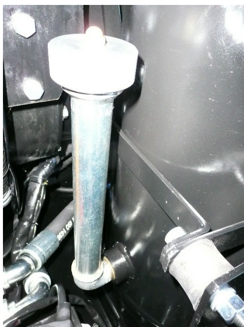
Figure 10.1-1 Checking the oil level in the compressor
