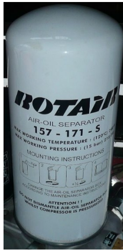
Figure 13.4-7 Oil separator filter
