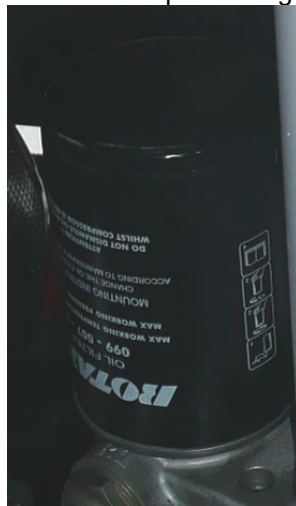
Figure 13.4-6 Compressor oil filter
