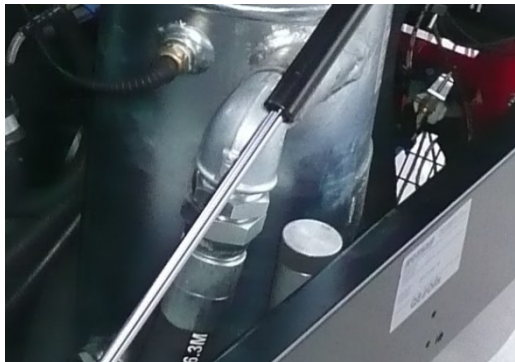
Figure 10.1-1 Checking the oil level in the compressor
