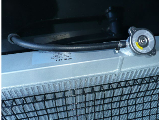
Figure 10.1-3 Checking the radiator cooling liquid
