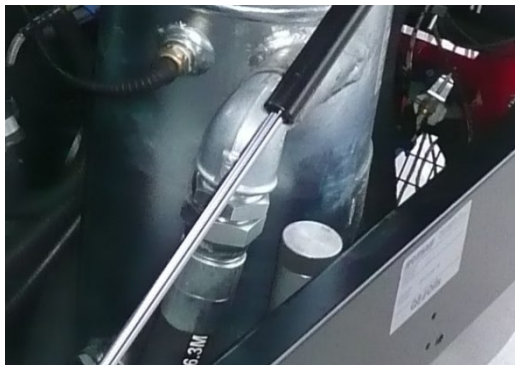
Figure 10.1-1 Checking the oil level in the compressor
