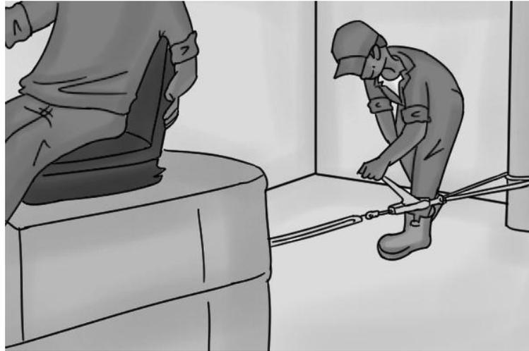
4. **Secure Load.** Make sure you secure the load that has been pulled so it does not move when the tension is released.
