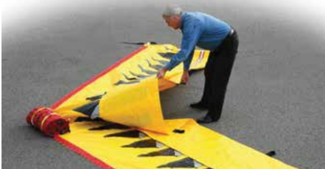
3 - Pull the material closer and smooth out the top fabric.
