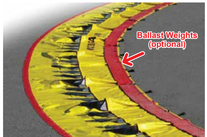
4 - Without ballast weights, the folds in the fabric are exposed to the wind. This opening may cause the Water-Gate to be lifted, jeopardizing the installation.
