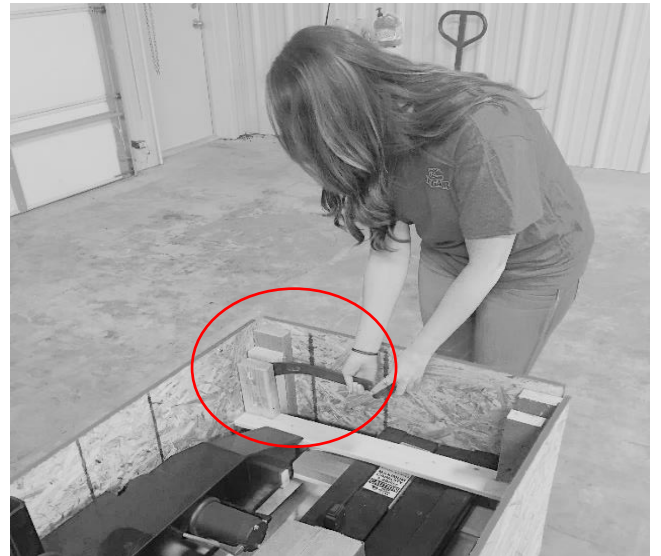
2. Using a pry bar and hammer, remove blocks holding pieces in place
