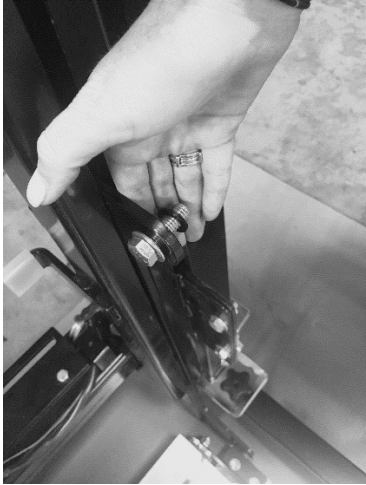
40. Place a bolt through the top tab on the carrier, with threads facing towards the outside of the liftgate frame. Place a nylon washer on the bolt once inserted through the carrier tab.
