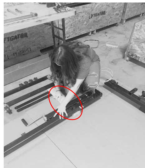
9. Place wooden blocks under both upright frame rails, making the frame rail sit flat on the floor
