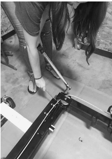
14. Tighten the nuts to 110 ft.-lbs.
