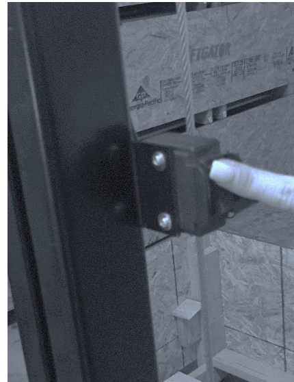
47. Press control switch up to raise platform. Check that platform lifts free of obstructions.
