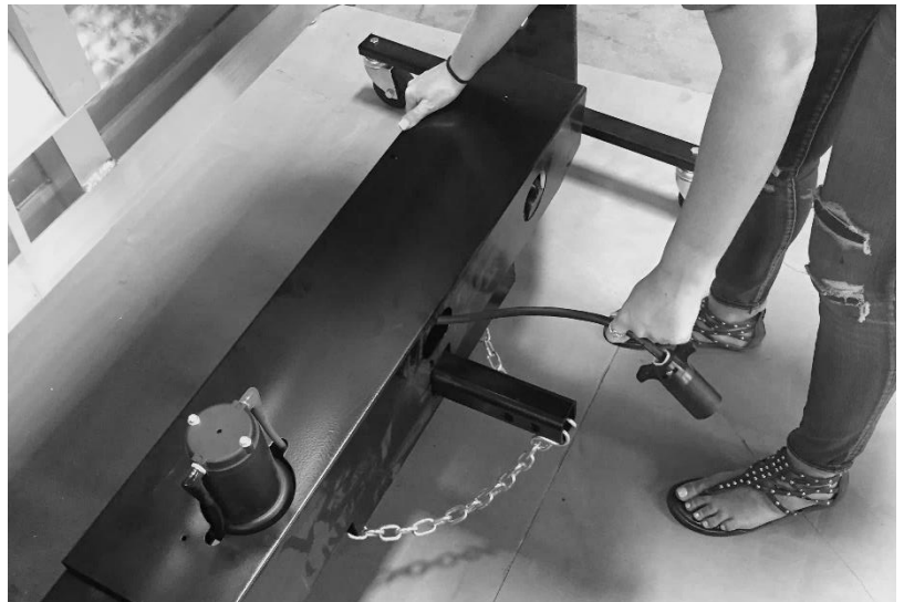
55. Install center crossmember cover, routing 7 pin connector through rear hole in cover.
