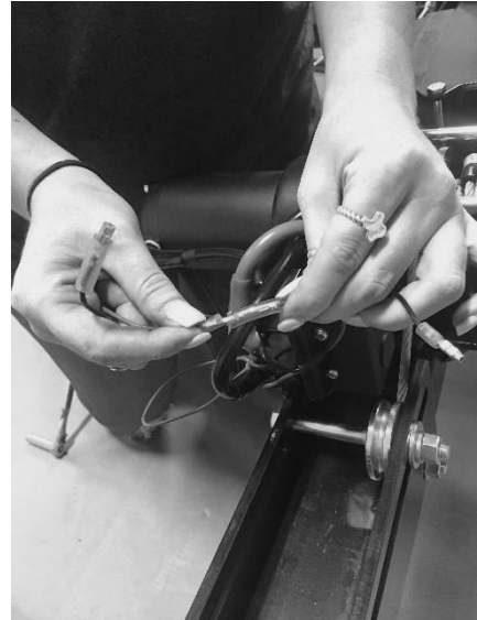
23. Insert the bullet connectors from the control switch harness to the solenoid wires. Green to Green, Black to Black.
