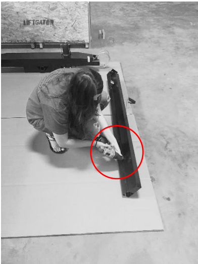
6. Remove the 4 screws on each upright frame rail which hold the cover in place, remove the covers.
