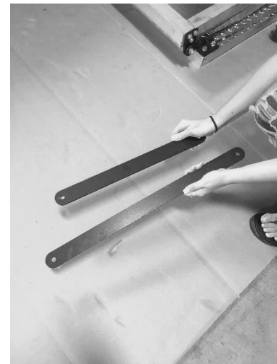
39. Match each set of links, one short with one long. Note the short link has a small hole on one end, a larger hold on the other.
