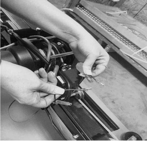
22. Identify the green and black control switch wires coming from the control switch harness and solenoid.
