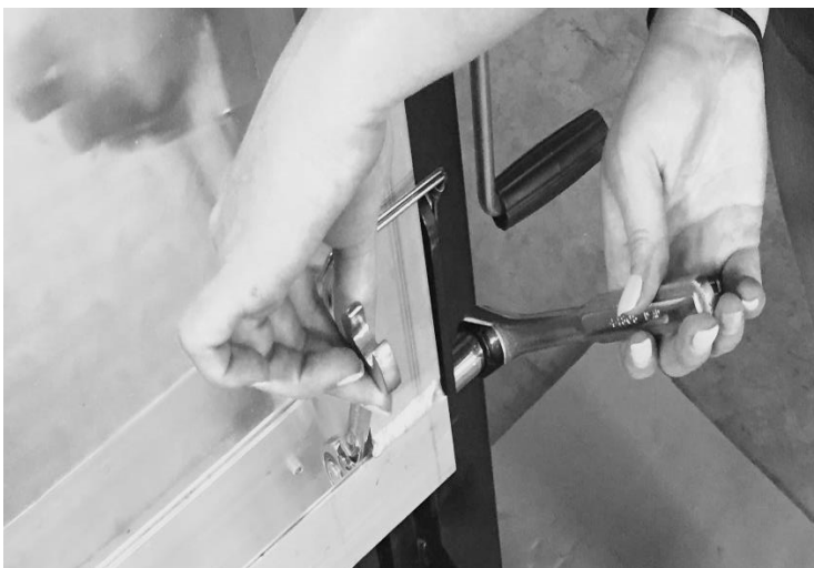
48. Tighten link bolts hand tight. Ensure that links can pivot with bolts tight.
