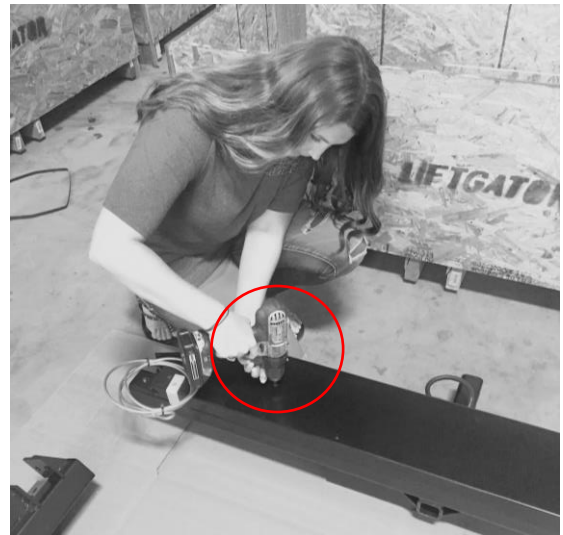
7. Remove the 4 screws on the crossmember which hold the covers in place
