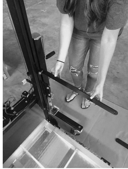
41. Place long link onto bolt, making sure nylon washer is sitting between carrier tab and link.
