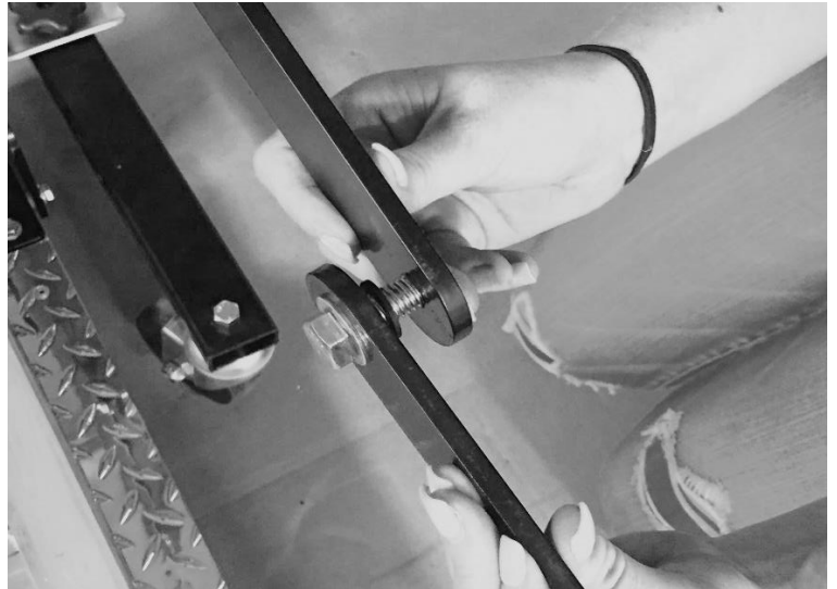
43. Place short link inside of long link, inserting bolt through hole on long link.
