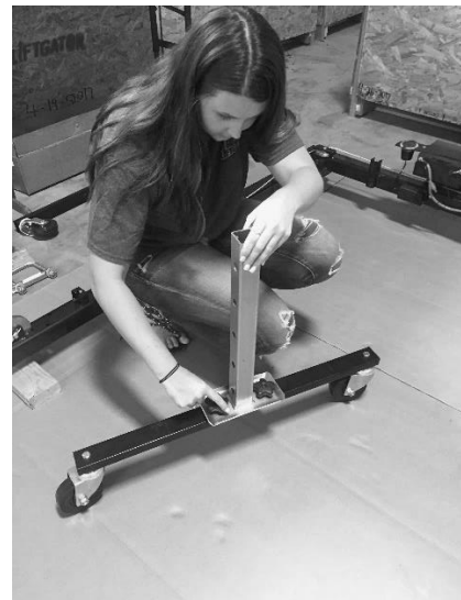
15. Place the support leg onto the skate studs and tighten the screw knobs
