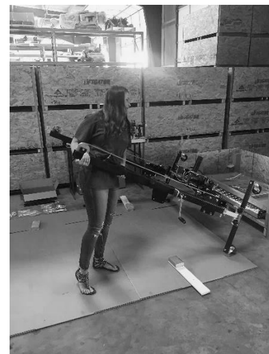
33. Tilt frame assembly and set frame upright.
