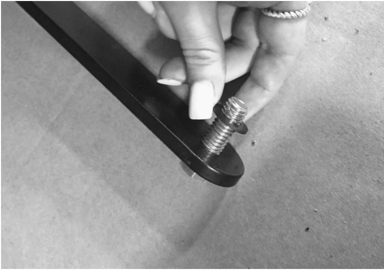
42. Insert bolt through large hole on short link. Place nylon washer over bolt once inserted.
