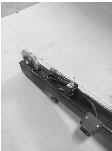
32. Ensure wires ropes are seated in all pulleys and cable sits free in bottom limit switch notch.
