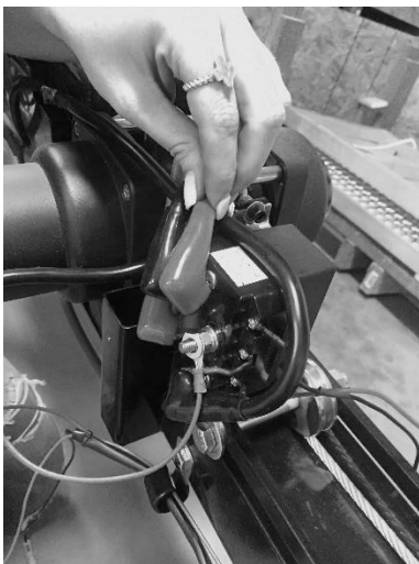
20. Place the control switch eyelet (red wire) and the positive battery cable (red cable) on the solenoid stud labeled "B+"
