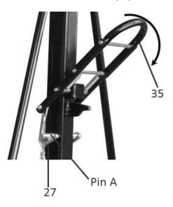
2. With the handling remaining, insert the Pin B (5) to the hole beneath Pin A. Then the height locked.
