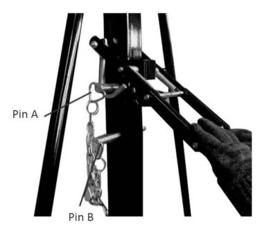
3. Pull the Safety Shaft (34) to release the hook on Pin A, lift the handle and hook up on Pin B.
