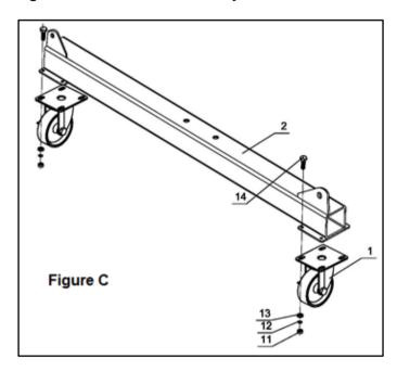
4. Apply grease to each Caster bearing.
