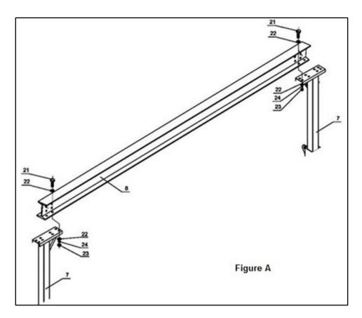
5. Attach Left Connector Plate A (9) and Left Connect Plate B (10) to I-Beam (8), using Bolts (21), Washers (22), Nuts (23), and Spring Washer (24).
