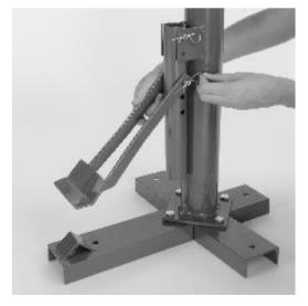
5. Slip the slotted press plate (#8) into the top of the post (#3).
