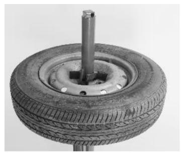
4. Once the tire is held securely in place, force demounting in between the tire and the rim. This should be done with the flat of the demount end against the rim. Pull the bar toward you across the tire to force the edge of the bead over the rim.
