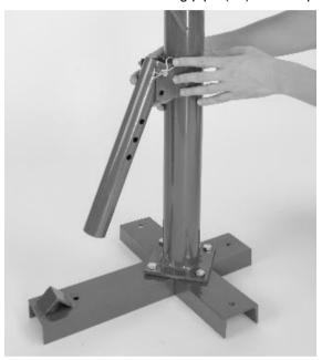
4. Connect the shovel (#7) to the casting pipe (#4) with the lock pin (#5) and hair pin (#6).
