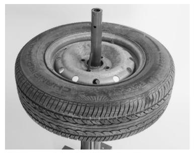
2. Place the slotted press plate (#8) over the center post.
