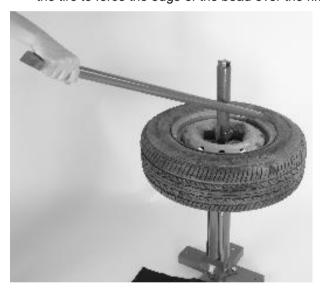
5. Work the bar all the way around the center post to demount the bead completely.
