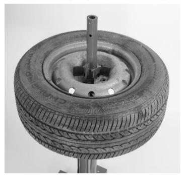
3. Screw the threaded rod (#9) onto the center post. Lock the slotted press plate into place by tightening by hand. Hand tightening should be enough but if you want a little more pressure, place the flat end of the dismount tool through the top of the threaded rod and use the extra leverage to tighten the threaded rod even more.
