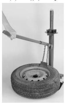
4. Push down on the mount/demount bar forcing the bead off the rim. If the bead does not come off all at once, turn the tire and try again in several different locations.
