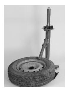
3. Insert the flat end of the mount /demount bar (#10) into the casting pipe (#4). Set the shovel (#7) on the tire against the edge of the rim. As you work with different sized tires you may need to adjust the shovel height. Adjust the shovel height by removing the pin and moving the shovel (#7) to the appropriate height and reinserting the pin.
