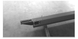
Step 2) Attach each Inner Vertical Post Assembly to the Crossbeam (#19). Secure with the 8 Bolts (#1), Washers (#2), Spring Washers (#3), and Nuts (#4)
