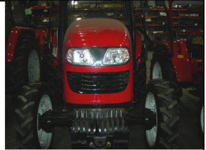
Figure 4-24 Combined Front Head Lamp Position
