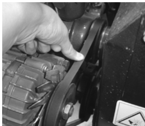
Figure 4-11 Fan Belt Tensioning Adjustment
