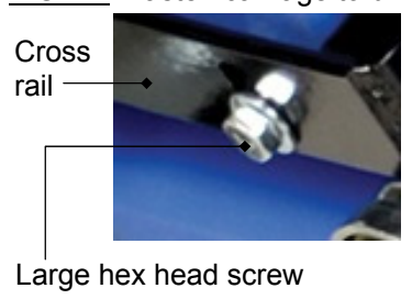
FIG. 1B: Fasten carriage to bin
