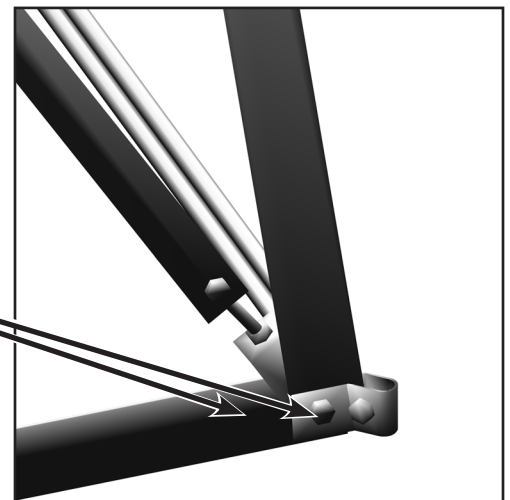
Anchor Bracket Installation
