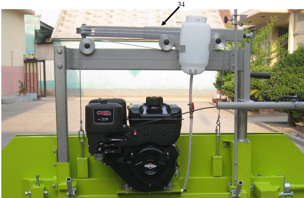
Figure M: Cable Route
