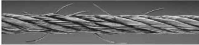
Cable with Broken wires (Replace Cable)
