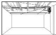
Plumb reference for ceiling installation
