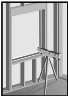
Squaring (window frame)
