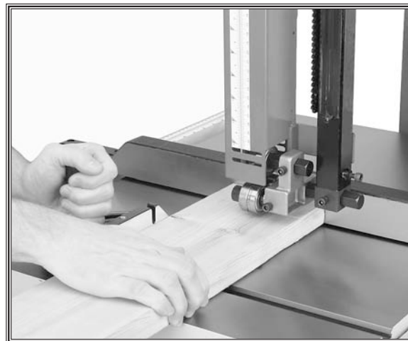
Figure 41. Typical crosscutting operation.
