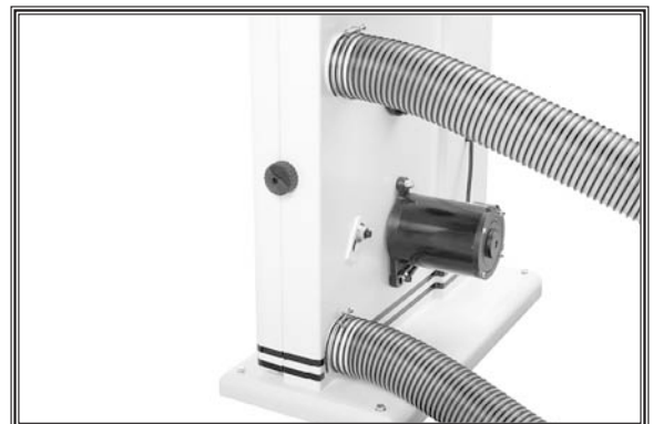
Figure 20. Dust port connected to dust collection system.
