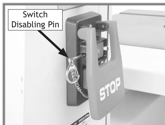
Figure 22. Switch disabling pin inserted into ON button.
