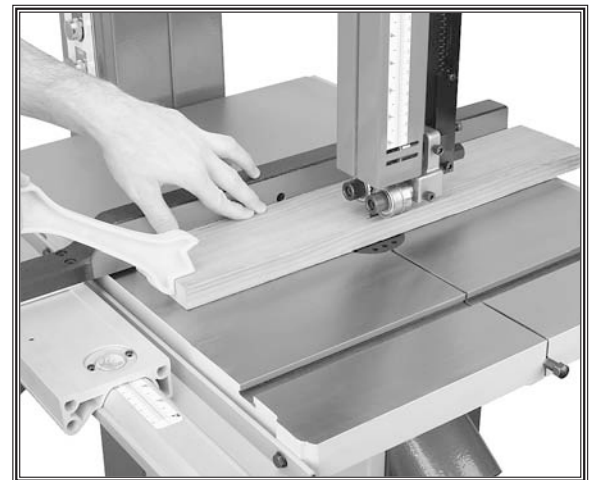
Figure 40. Typical rip cut.
