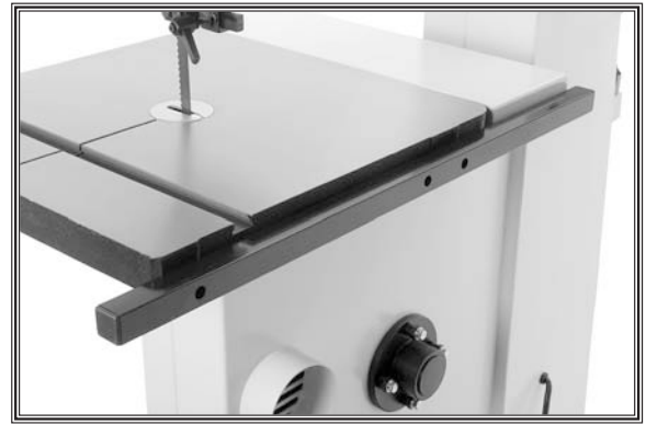
Figure 13. Rear fence rail attached to table.
