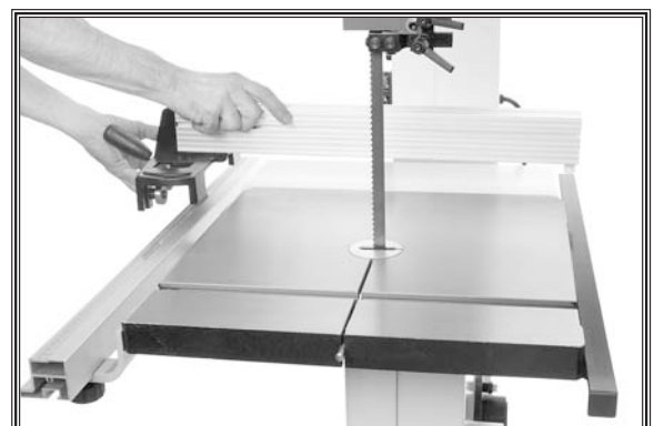
Figure 16. Installing fence onto rails.
