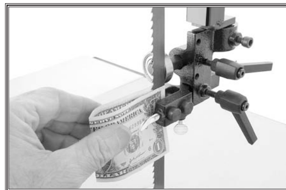
Figure 30. Blade guides against both sides of blade.
