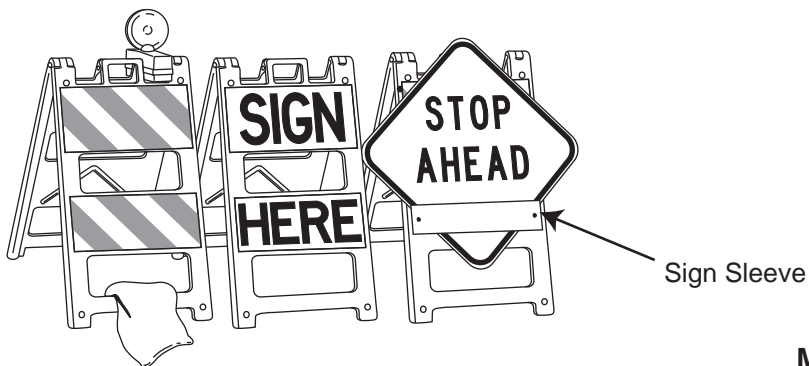
With the addition of a sign sleeve, the Plasticade barricade becomes a sign stand (NCHRP Certified)
