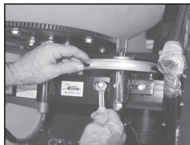
Step 7 Slide drum on frame. Then install pinion housing. Line up front of pinion with front large gear (Note: Do not position pinion to far forward, so gear will dig into drum.)
