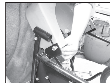
Step 9 Install ring gear guard with 3/4" hex screw.
