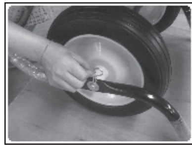
Step 4 Put washers on the axle, then fix R clips into holes.
