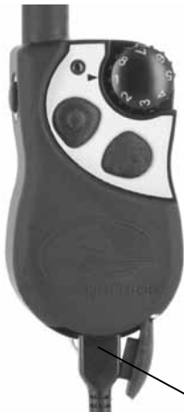
CHARGER CONNECTOR PLACED IN THE REMOTE TRANSMITTER CHARGING JACK
