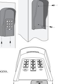
**IMPORTANT:** Transmitter must be placed <u>exactly</u> as shown, and against the bottom of the keypad in order for the 'learning' process to work correctly.
