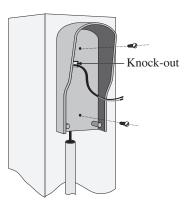
**Step 2**: To hard-wire the keypad - strip the wires back 3/16" and attach the wires to the terminal block marked OUT COM on the keypad control board as shown to the right making sure to obey polarity (+ -). Connect the other end to the opener's control board as shown in Control Board Connections section below.
