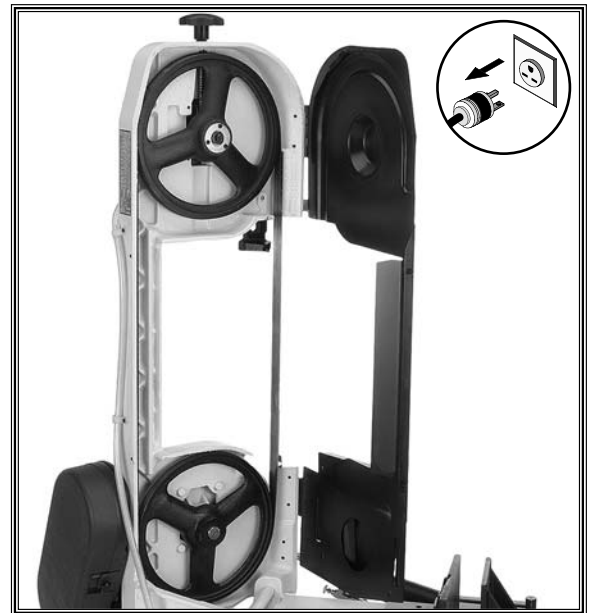
Figure 27. Bandsaw ready for blade tracking.
