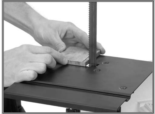
Figure 4. Always use the table for freehand cutting and keep fingers clear of blade.
