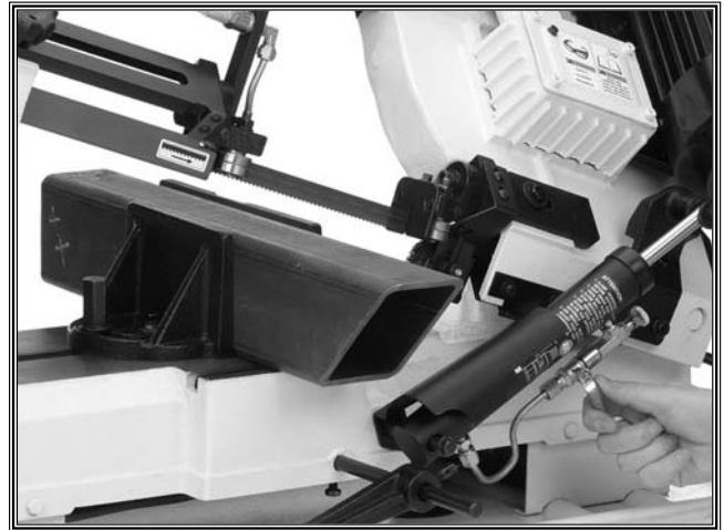
Figure 5. Always start the saw with the blade clear of the workpiece.
