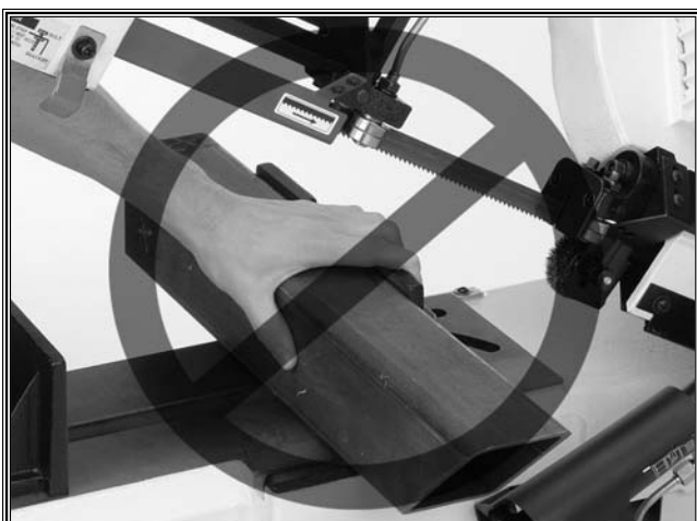
Figure 3. Never hold the workpiece by hand.
