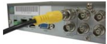
Plug RCA cable to BNC connector
