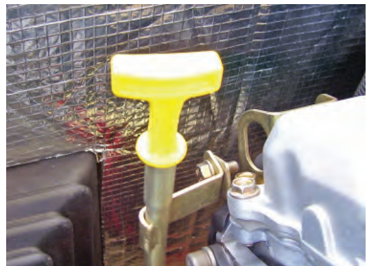
Figure 4.3 — Oil Dipstick and Fill, 12, 14, 16, 17 & 20kW
